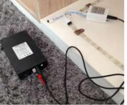
6. Plug in the end of the power cord to the battery.
