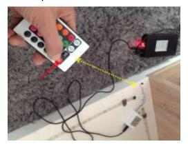
11. If the LED lights do not work, turn the signal receiver end to the other side, and plug in again.
