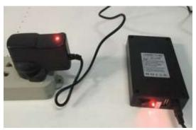
9. Keep on recharging till the power supply lamp show green color and battery is full. (It will take 6 – 7 hours)
