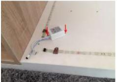
3. Connect the signal receiver to the strip (make sure that the arrows are facing each other).
