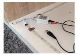
5. Plug in the USB end of the connecting cord to the battery.
