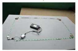
2. Assemble the remote control signal receiver onto board, using the given screws.
