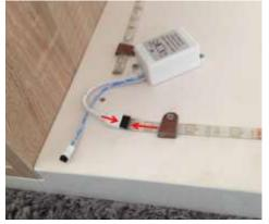
4.Plug in the round end of the connecting cord to the signal receiver.
