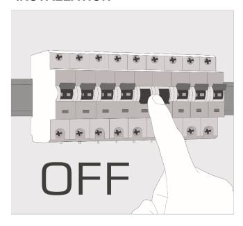
1. Ensure power is disconnected from the circuit and there is no risk of accidental reconnection before starting installation
