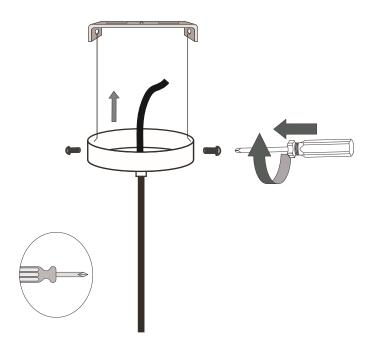
5. Reattach the Ceiling Rose to the Mounting Bracket using the bolts removed in Step 2.
