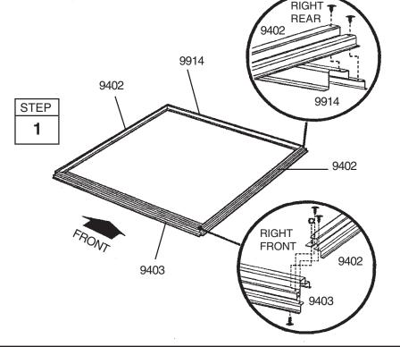
**2** Measure the floor frame diagonally. When the diagonal measurements are equal, the floor frame is square.
