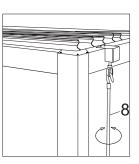
8 Install onto concrete pads or cemented paving slabs
