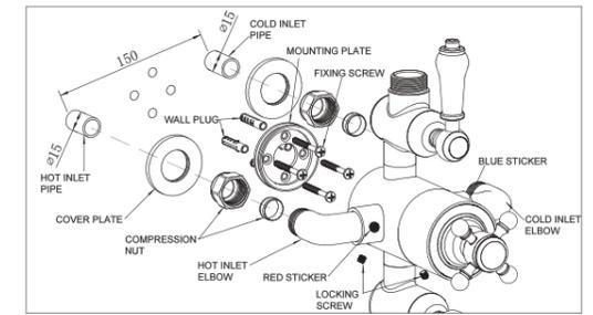
The valve should be installed in accordance with the water bye-laws. For further details refer to the latest copy of Water Bye-laws guide or your local water authority.
