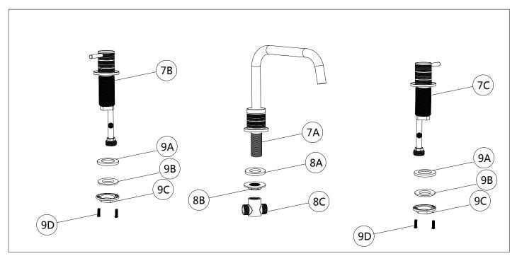
Thrust the hot and cold control valves through holes on bathtub. From underneath basin, secure valves(7B & 7C) by placing Rubber Washer(9A), Metal Gasket(9B) and locknut(9C) onto the body. Fasten the two screws(9D) by using tool.
