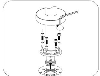
Slide down the base(2)until it reaches the floor. Waterproof adhesive is recommended to be applied.
