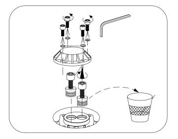
Fix the G3/4 connectors(9) to inlets of the body(8). Thrust the body over floor screws(11) and fasten with steel plate and nut. Connect the body(8) with hot (LHS) and cold (RHS) water pipes using thread seal tape.
