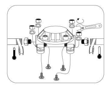
Fasten the holder(4) with the body(8) by fixing screws(3).
