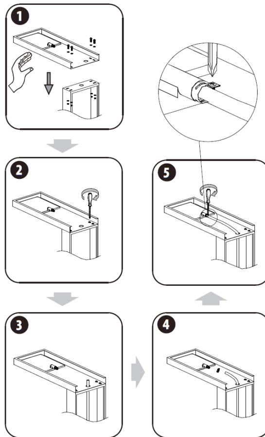
Connect the water supply pipes to the flexi-pipes on the rear of the panel, ensuring hot is on the left and that the seals are fitted, then tighten the nut.
