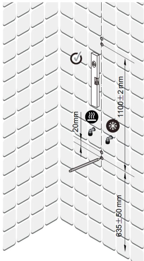
If drilling into tile, it is recommended to tape the wall to prevent the drill from slipping.
