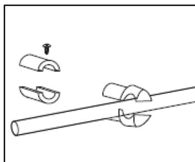
6. Once both parts of the rail brackets are fitted, align and push the rail brackets on the radiator onto the wall brackets secured to the wall, ensure that there is equal distance from the wall to connect to the supply pipes. Secure each bracket set with the grub screw provided (insert through the slot in the bracket), be sure not to overtighten.
