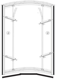
Align assembly on the tray to position frame holes over drilled holes in tray
