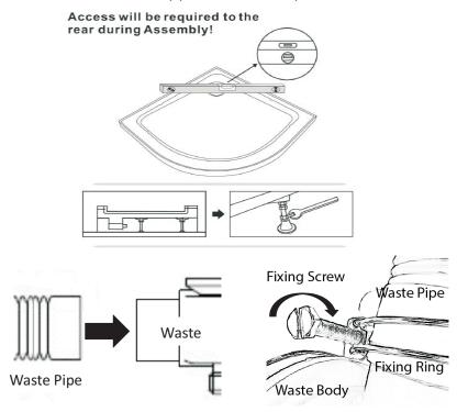
Before installating the tray, connect the waste pipe (X) and fixing ring to the waste body, once connected tighten the ring using the screw.
