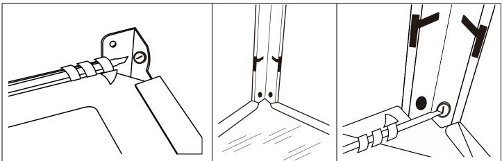
**STEP 6:** Unscrew the eight M5 Screws and Washers preassembled on top of the MAIN BODY (K). Place the bottom of the SUPPORT BARS on the top of the MAIN BODY. Make sure to match the top of the MAIN BODY with the on the SUPPORT BAR. Match the threaded hole and fix each connection with 2pcs M5 SCREWS and WASHERS (BB)
