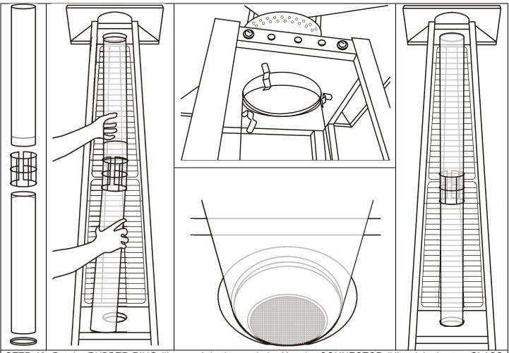
**STEP 10:** Put the RUBBER RING (I) around the burner hole. Use the CONNECTOR (H) to join the two GLASS TUBES (G). Hold the whole glass tube assembly carefully. Insert the top end into the bottom hole of the FLAME SCREEN and slide through it as far as possible. Keep the whole glass tube assembly vertically and sit it on the RUBBER RING (I).
