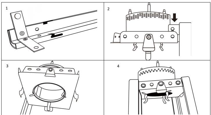
**STEP 4:** Attach the FLAME SCREEN (B) to the top of assembled SUPPORT BAR and fix using two M5 SCREWS and WASHERS (BB) (See Figure 1, 2). Repeat this step to connect the FLAME SCREEN (B) to other 3 assembled SUPPORT BARS. (See Figure 3, 4)
