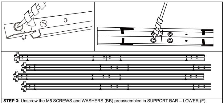
Connect the UPPER SUPPORT BAR (E) to the LOWER SUPPORT BAR (F) and fix them together using the SCREWS and WASHERS. Repeat this step for all 4 SUPPORT BARS.
